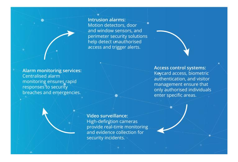
By integrating these elements into a single centralised alarm system, school facilities managers can monitor security events in real-time, receive immediate alerts, and coordinate responses more effectively.
